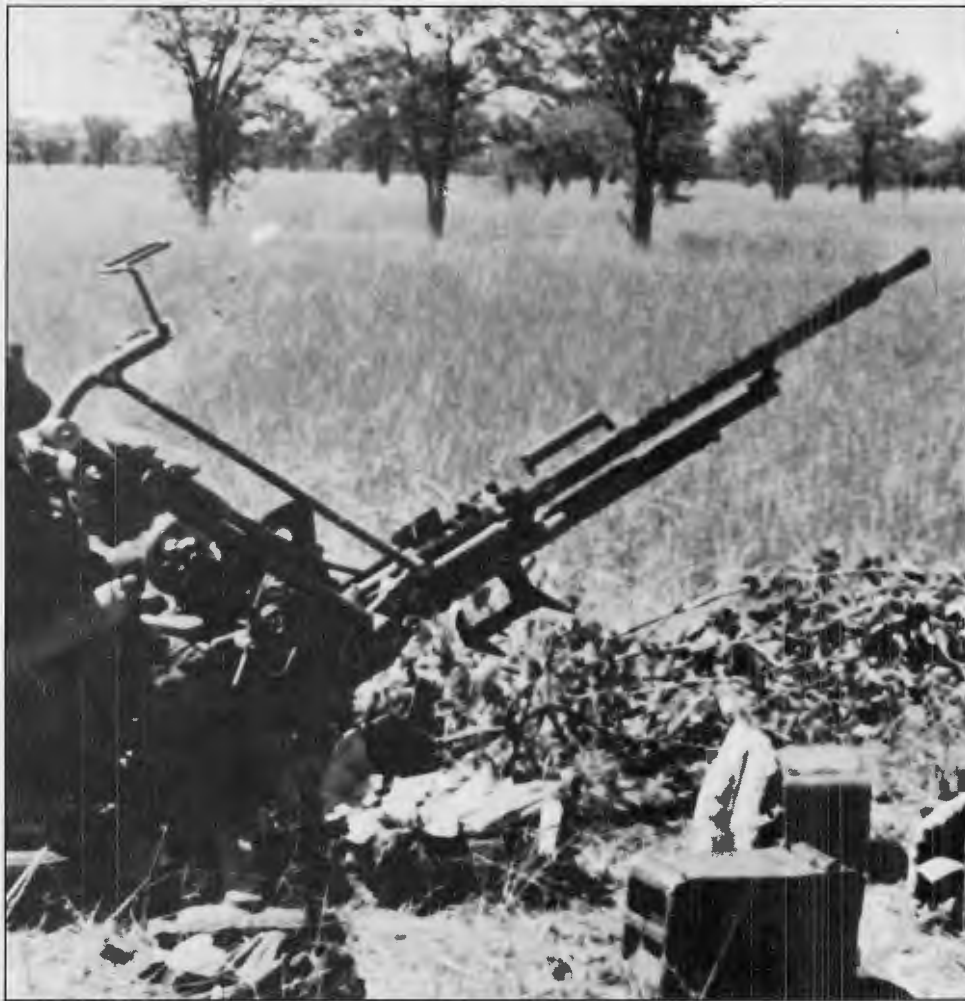
South African officers examine a Soviet-made 14.5mm heavy machine gun captured from the terrs.
